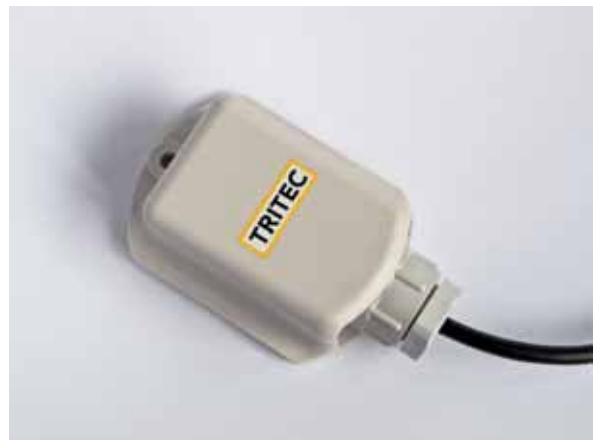
TRITEC outside temperature sensor Pt1000
