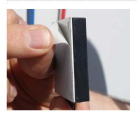
Attach the STS to the target measuring point. After removing the protective sheet from the adhesive strip, the STS easily attaches to the clean surface of the solar module.
