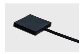
The surface temperature sensor (STS) is designed for temperature measurements on surfaces. Installed at the back of a solar module, the STS measures the module's temperature. The temperature of the solar modules is crucial for their output which decreases by 0,43 % per Kelvin with increasing temperature (typical value for mono- and polycristalline modules).
