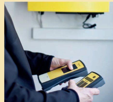
Wireless transmission of the data from the TRI-SEN to the TRI-KA.
