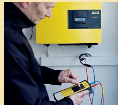
Measure the open-circuit voltage and the short-circuit current with TRI-KA and determine the current/voltage characteristic curve of the system.
