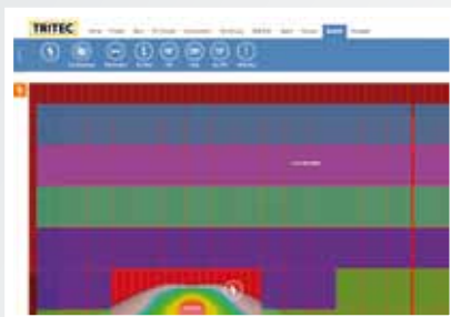
Step 5 Determine string connection graphically for circuit diagram.
